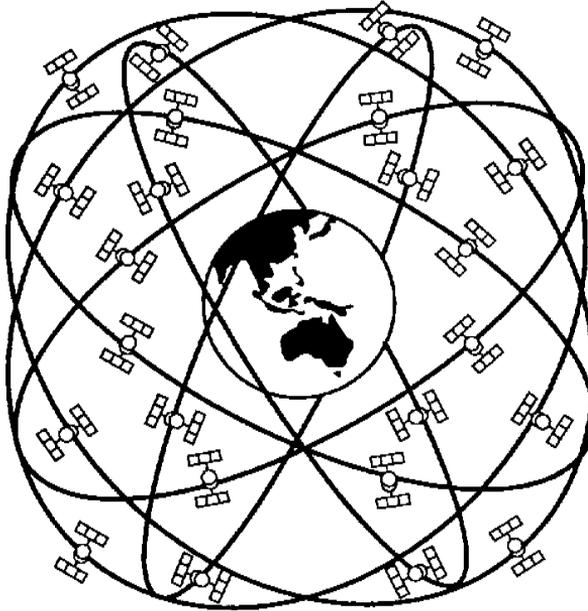
Each satellite whizzes around about 20 200 kilometres above the Earth's surface. That's about the same distance as from the South Pole to the North Pole, the long way ... but straight up! This incredible altitude, and the birdcage pattern of orbits allows us to 'see' between four and ten satellites at any time, from anywhere on the globe.
