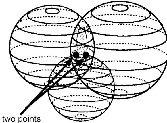
This is more like it. It restricts the number of possible positions to just two, (the intersection of three spheres is two points.) Panic stations! Which one is right?
