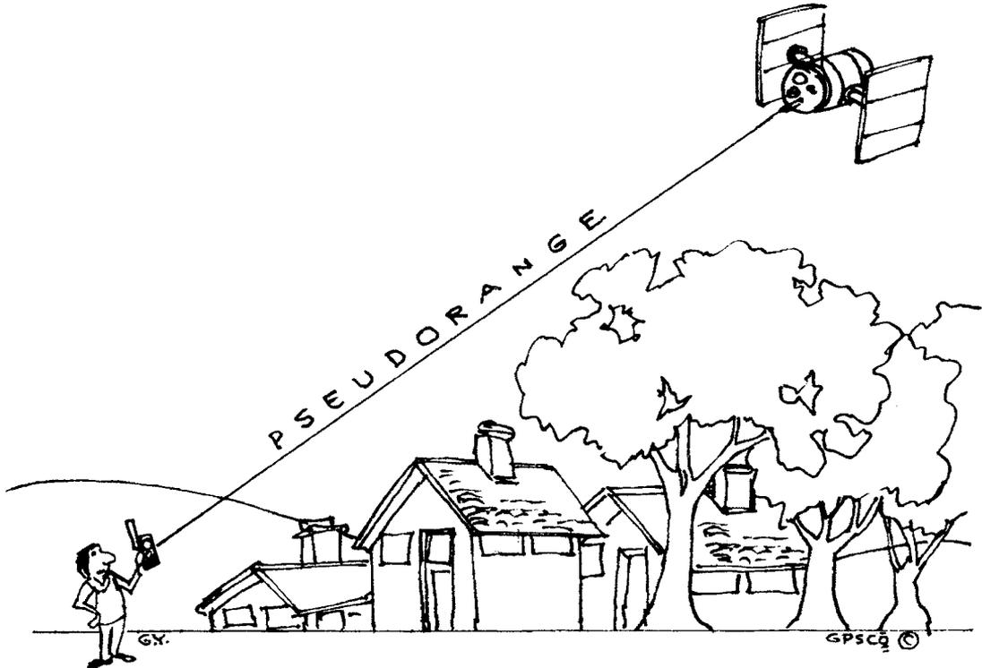
Signals from GPS satellites are microwaves which travel at the speed of light - that's about 300,000 kilometres per second - quite a bit faster than a car. But the formula still holds.
